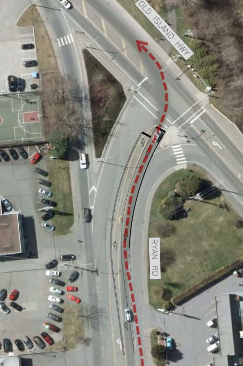
FIGURE 24. RYAN ROAD / OLD ISLAND HIGHWAY WESTBOUND QUEUE JUMP LANE CONCEPT
